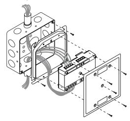
**SIGA-MCC1** and **SIGA-MCC2**: mount the UIO motherboard inside a suitable EDWARDS enclosure with screws and washers provided. Plug the SIGA-MCC1 or SIGA-MCC2 into any available position on the motherboard and secure the module to the motherboard with the captive screws. Wiring connections are made to the terminals on the motherboard (see wiring diagram). UIO motherboard terminals are suited for #12 to #18 AWG (2.5 mm² to
